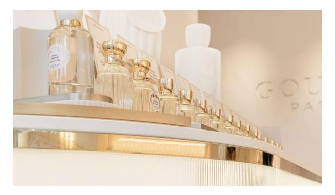
The design also demanded 8cm strips of Raywal 45 glass to be shaped over the lighting strip on the curved central counter, while Ressource lime plaster was hand-applied to every wall and the ceiling.
