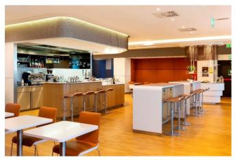
For this reason, not only the central food counter and the suspended shelfs but also the high tables, the laterally placed main bar and the partitions were all made of **HI-MACS®**. They were designed with the non-porous Solid Surface material in **Alpine White**.
