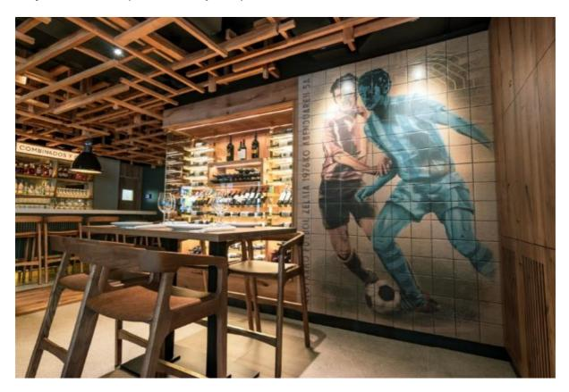
Sublime, the Group Concord company in Mallorca tasked with designing the murals, explains the sublimation process performed on HI-MACS<sup>®</sup> as a complicated technique, by which **digital prints were transferred in a gaseous state to the solid surface**, by applying controlled pressure and heat in special kilns.
